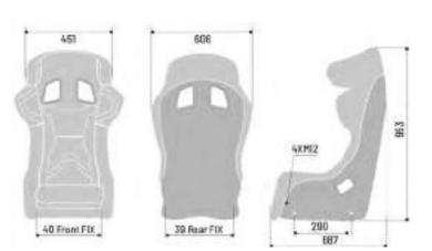
HOMOLOGATION: FIA 8855-2021 MATERIAL: FIBERGLASS HRS: YES WEIGHT (GR): SHELL: 9700 / SEAT: 12000
