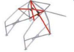
Racing start kit is proposed to upgrade the existing Appendix J roll cages. This kit is composed of 6 tubes to build up the cross reinforcement for the roof and the main roll bar, complete with reinforcement gussets.
