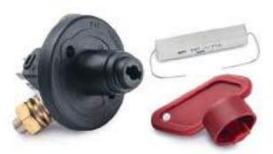
Battery master switch with rotating lever. Instant disconnection of all electric circuits. Provision for remote control Complies with FIA spec. Suitable for 6, 12 and 24V systems, rated at 100A continuous.
