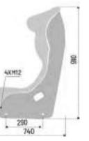
HOMOLOGATION: FIA 8855-1999 MATERIAL: CARBON-KEVLAR PRE-PREG HRS: NO WEIGHT (GR): SHELL: 5300 / SEAT: 6000
